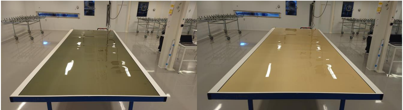
Figure 1: Demonstrator of a \text{WO}_3\text{-NiO} (CL70) EC device (5000 x 1500 mm 2 ) L5528: left side in the dark state, right side: in bleached state
