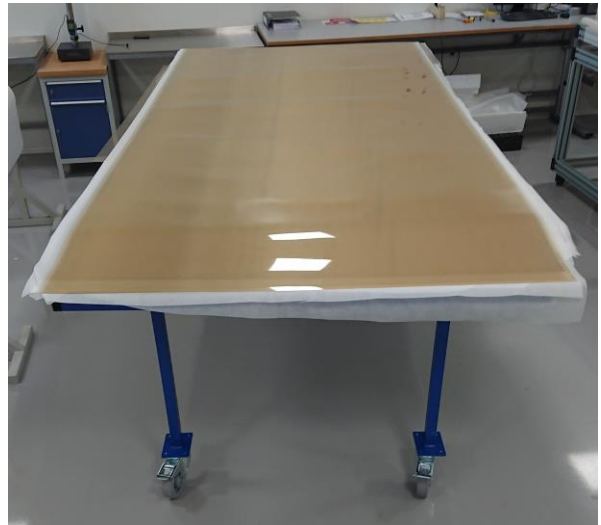
Figure 3: Electrochromic film \text{WO}_3/\text{NiO} CL70 L5528 1500 mm x 5000 mm after lamination before cutting and bus bar application.
