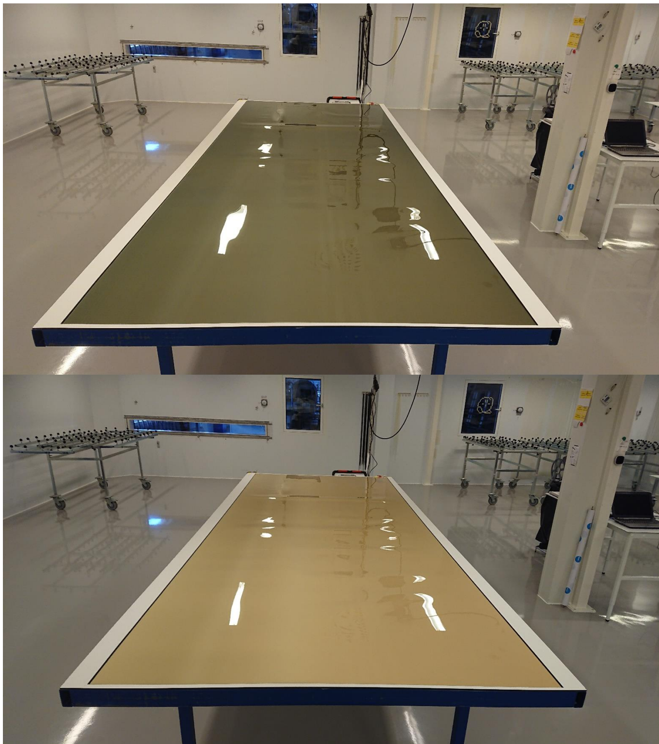
Figure 4: Demonstrator of a \text{WO}_3\text{-NiO} (CL70) EC device ( 1500 \times 5000 \text{ mm}^2 ) L5528: picture on top in the dark state; lower picture in bleached state.
